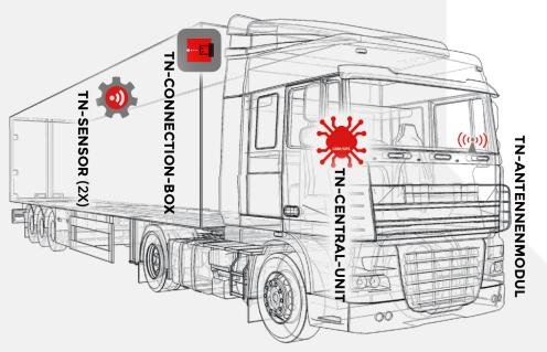
Audio is registered by microphones and detected in the central unit by means of artificial intelligence. Two sensors are fixed on the left and right sides of the tarpaulin with strong magnets or screws.
