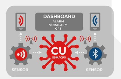
Trained with tens of thousands of real cuts, our Artificial Intelligence (Al) detects every cutting noise on the tarpaulin by means of audio recognition. Cuts can be detected even when there is loud background noise or attempts at manipulating the device.
